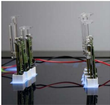
Figure 3 – ShapeClips placed on LCD screens, which are used to control their heights.
