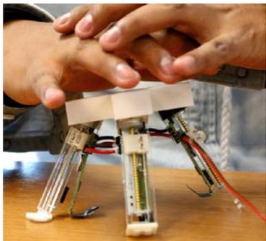
Figure 4 – demonstration of actuation ShapeClips by blocking natural light.
